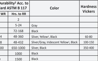
2. The hours listed are for white corrosion (WR) and red corrosion (RR). The hours refer to optimal combination of coating layer, coating thickness, passivation type and the type of sealing that we use. Please note: the standard coating, which is common in the standard fasteners market is "White Zinc" coating with white corrosion resistance of 6 hours . and "Yellow Zinc" coating
