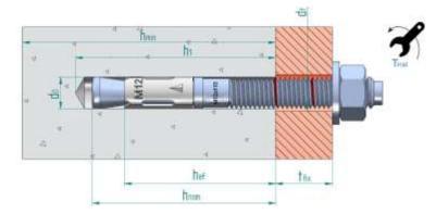
Reduced embedment depth (sizes M8, M10, M12, M16 and M20)
